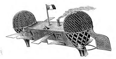
containing the motive power, and the propelling is performed by oars and a screw.
